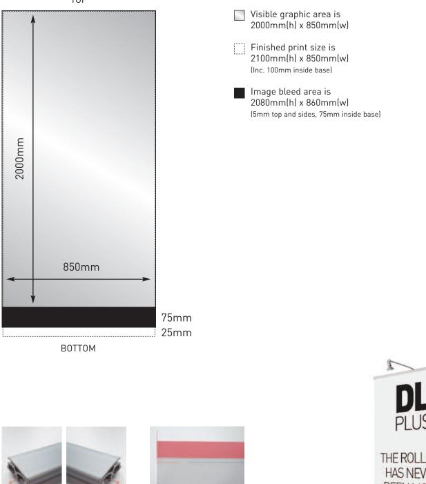
Ensure graphic is fully inserted to the graphic rail inner shoulder and positioned centrally.
