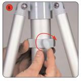
Position the clamp near to the top of the stay set and tighten the thumbwheel to secure.
