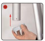
Slide the pole clamp over the telescopic pole.
