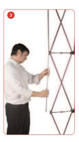
Attach the magnetic bars to the pop-up frame nodes
