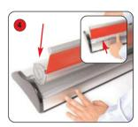
Load the cassette into the base and close the snap retainer to secure.
