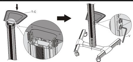
Insert the DVD shelf to the required position along the column rails. Secure it by tightening screws with an Allen key.
