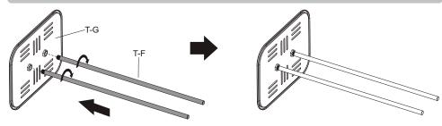
Tighten the support rods to the camera shelf.
