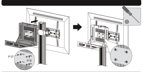
Attach the laptop cabinet to the connecting piece on the universal plate using the appropriate screws. Tighten all screws with a proper phillips screwdriver.
