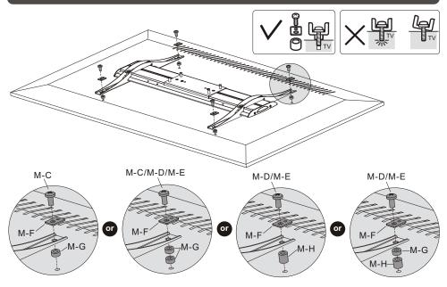
Note: Choose the appropriate screws, washers and spacers (if necessary) according to the type of screen.
