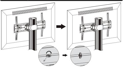
Insert the cable clamps horizontally into the plate slots, then turn the cable clamps to the vertical position to secure them.
