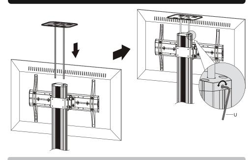
Insert the support rods to the required position along the column slots and tighten both screws to secure the camera shelf.
