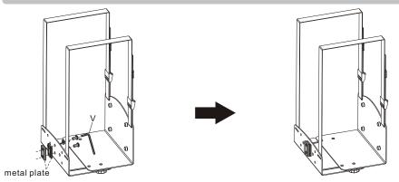
Attach the removed metal plates to the CPU holder using the removed screws. Tighten all screws with an Allen key.
