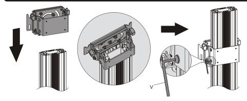
Insert the support plate along the column rails to the required position and tighten all screws with an Allen key.
