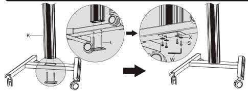
Attach the column to the assembled base using the connecting piece, secure them with the appropriate screws. NOTE: Lock the brakes on the casters to avoid any sudden movements during installation.
