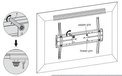
Install the two nuts (the removed in previous step) on the upper pins and leave a 5mm space to the universal plate.
