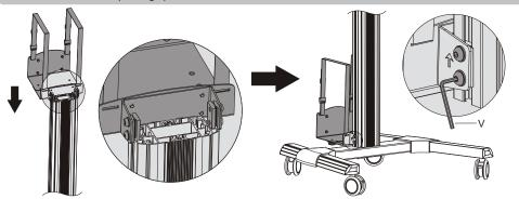
Insert the CPU holder to the required position along the column rails. Tighten all screws to secure it with an Allen key.
