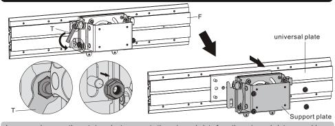
Loosen and remove the nuts in order to separate the universal plate from the universal plate assembly.
