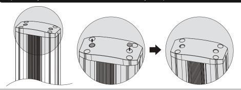
Remove two plastic caps for the camera shelf installation.
