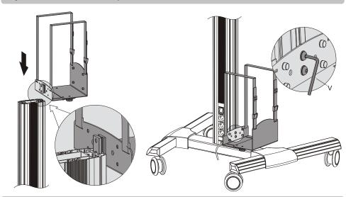
Insert the CPU holder to the required position along the column rails. Tighten all screws to secure it with an Allen key.
