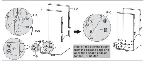
Attach the connecting piece to the CPU holder using the appropriate screws. Tighten all screws with an Allen key.
