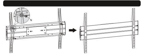
Adjust the adapter brackets to align with display mounting holes, then tighten all screws using a proper screwdriver.
