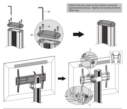
Lift the display carefully and hook the display onto the support bracket. Place the lower nuts and use a wrench to tighten all nuts.
