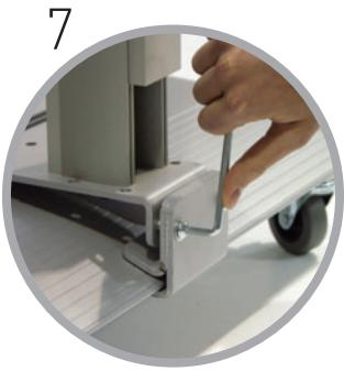
Position column centrally within central channel and fully tighten both clamp bracket screws.
