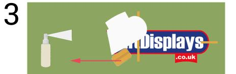
For larger stickers use application fluid to wet the surface. Using a squeegee flatten the sticky side onto the surface from the centre outwards
