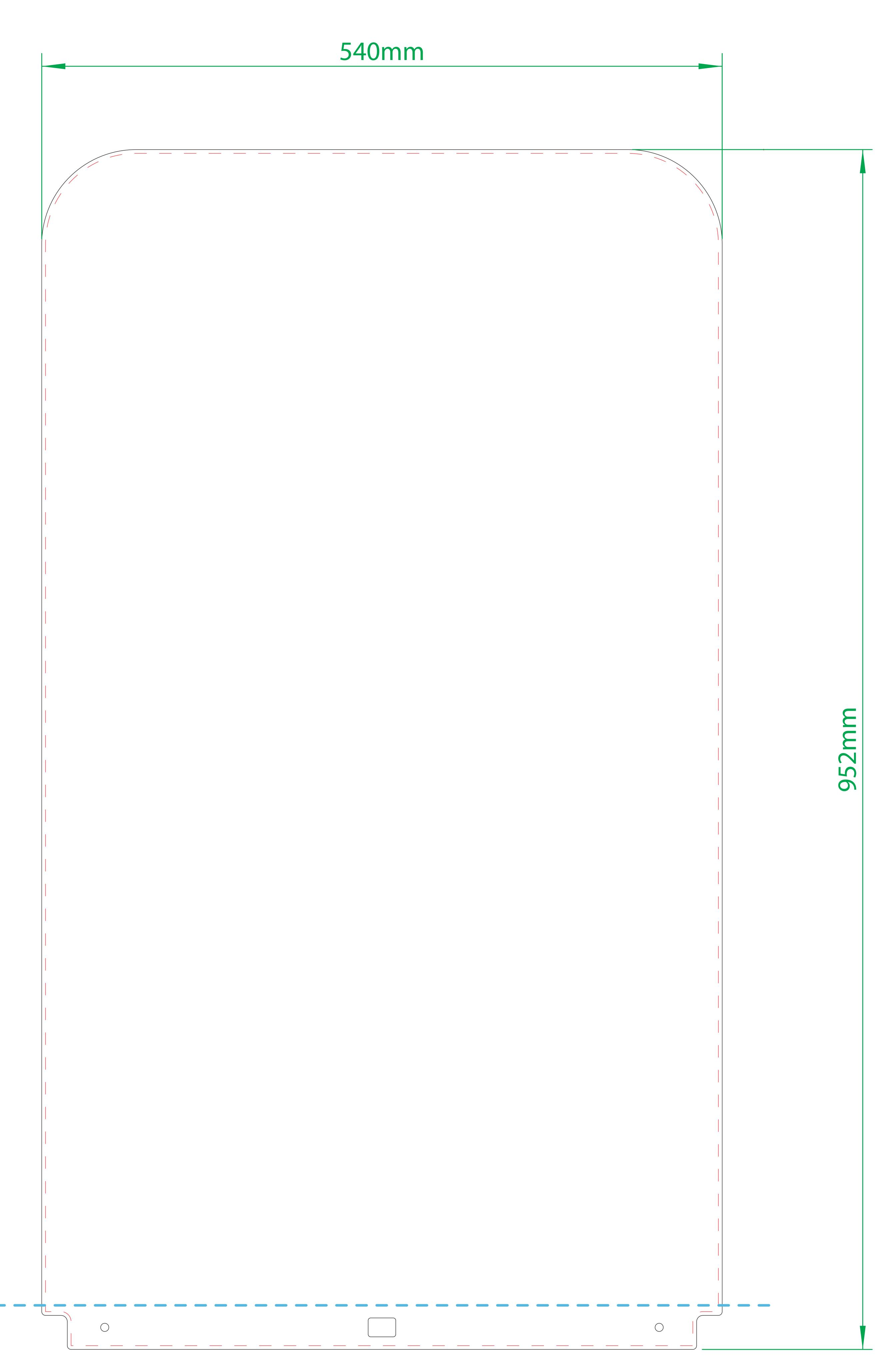
PLEASE NOTE: THIS AREA UNDERNEATH THE BLUE DASHED LINE IS NOT VISIBLE WHEN PANEL SLOTS INTO BASE.
