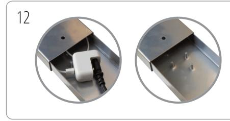
Carefully position and slide top support plate onto end of bottom support plate, ensuring the internal cables do not interfere with this assembly. Repeat stages 11 and 12 for remaining iPad holder.
