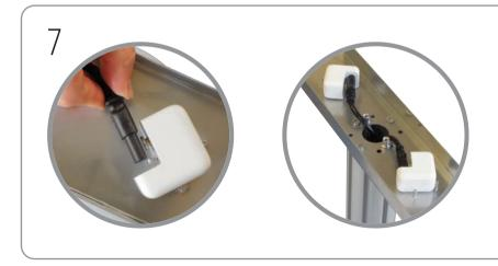
Plug one figure 8 head into a USB Power Adapter (supplied with Apple iPad) and position into retaining pins. Repeat for remaining power lead and adapter.
