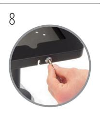
Unlock each iPad enclosure by inserting key into security lock and rotate 'QUARTER TURN ONLY' clockwise or counter-clockwise through 90 degrees, which releases the locking pin. Return key back to original position to remove.
