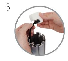
Plug figure-8 head into USB Power Adapter (supplied with Apple iPad).
