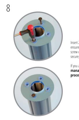
Insert 2 diametrically opposite screws to ensure holes are aligned. Fully tighten 1 screw using hex key provided and once secure, remove opposite screw.
