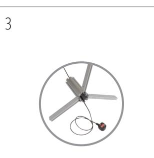
Feed figure-8 head of power lead through bottom of post and profiles assembly, leaving approximately 1m of cable at bottom.
