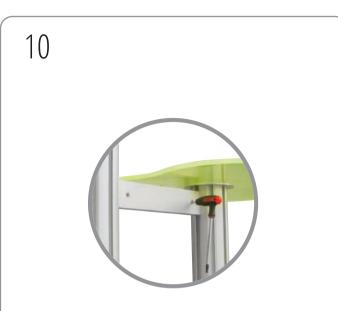
Position remaining 220mm profiles between posts near underside of Podium tops. Insert clamps into channels and secure by tightening grub screws.
