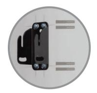
For brick/concrete walls, use 8mm masonry bit to drill 4x holes. Insert 4x rawl plugs and secure back plate of mount using screws and washers supplied.
