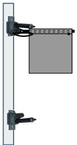
Install the bottom bracket on the marked line using Step 1-5,
