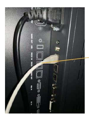
The Third RS232 cable is connected into the 'RS232 IN' input on the screen. This completes the daisy chain and connects all the screen's together, ready for the multimedia software.
