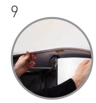
Align slots and channel in the underside of table top with hubs and graphic, and carefully lower into position.
