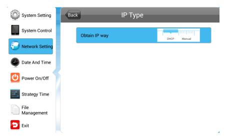
To set a static IP address, press the "RIGHT" navigation button to move the slider to "Manual". This will open up four new fields; Local ID, Subnet Mask, Default Gateway and DNS. Once you have inputted your information into these fields navigate to and select "Back". The system will ask to if you want to reboot the screen so that the changes can take effect, select "YES".
