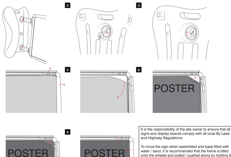
To move the sign when assembled and base filled with water / sand, it is recommended that the frame is titled onto the wheels and pulled / pushed along by holding the top corner of the frame . The handle on the base is not to be used when the base has been filled with water/sand.
